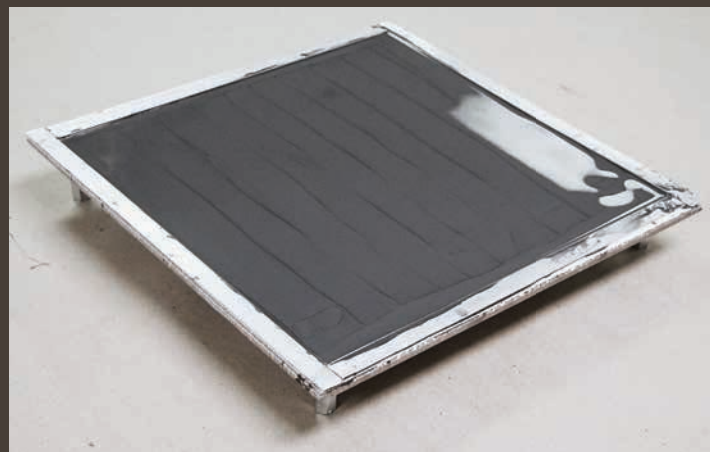
Modified silicone cast onto tile: thickness is controlled by volume pour
