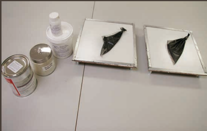
Components and mixtures prepared for casting on to ceramic tile into sheets
