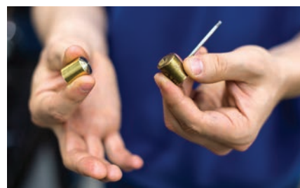
HAMMER HELPER: New parts made by Loudon Blake '17 (above) in the fabrication lab in Rettner Hall are designed to replace pieces of a keyboard that were originally custom made about 40 years ago.
