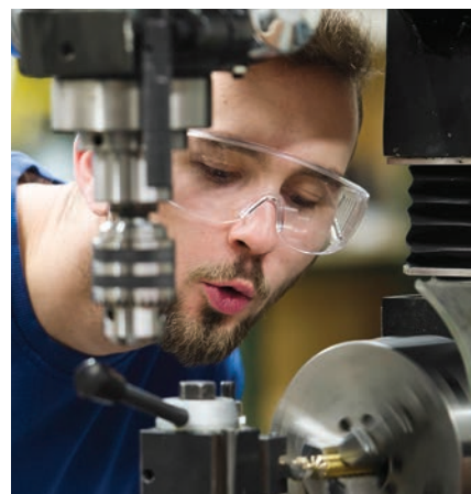
BRASS ATTACKS: Jim Alkins works with Ben Martell '19 to mill brass replacement parts for a practice keyboard used to teach students how to play the University's carillon.
