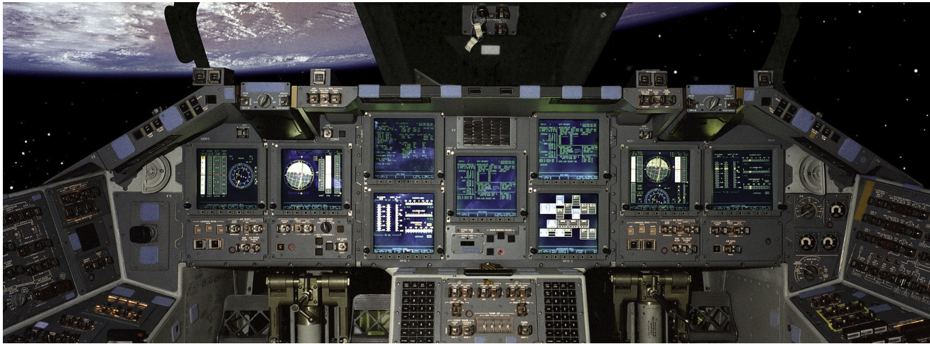
Figure 1: The cockpit of the Space Shuttle Atlantis while in orbit around Earth on mission STS-101. This image shows the new touchscreen panels and displays that were installed.
