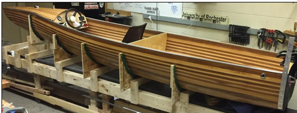
Figure 5: URSS' 2017 entry after completion of cedar strip, fiberglass, inner-deck, center console, and lid
