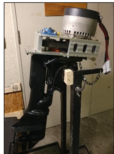
Figure 7: Modified 1965 Johnson-Evinrude 5.5 hp with 1.78:1 belt drive system
