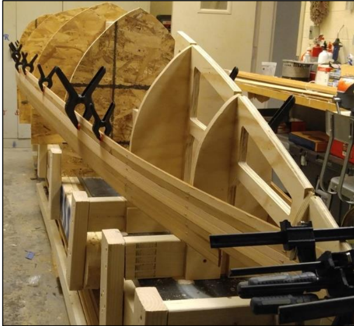
Figure 6: Cedar strip glue and staple application mid-process, note that the birch plywood stringers are permanent, while particle board stringers are temporary
