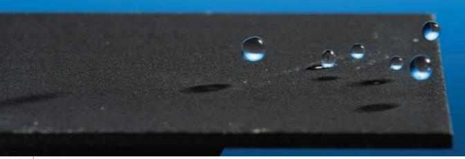
BOUNCING: Water droplets bounce off a surface that has been treated with a new laser-based process that makes metals water-repellent.
