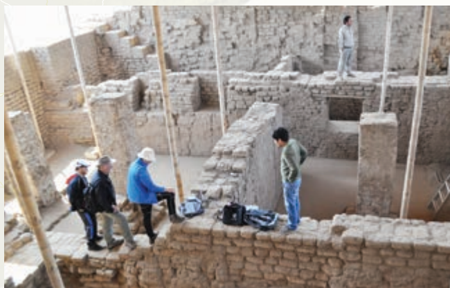
AT WORK: Perucchio (second from left) and Peruvian colleagues measure the dynamic response of adobe walls in Huaca de la Luna.
