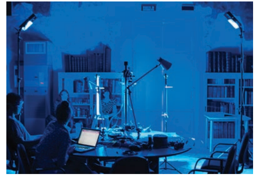
COLORFUL VIEWS: The equipment—set up here in Vercelli—exposes manuscripts to different wavelengths of light, including blue, red, and ultraviolet, in an effort to recover as much lost text as possible.
