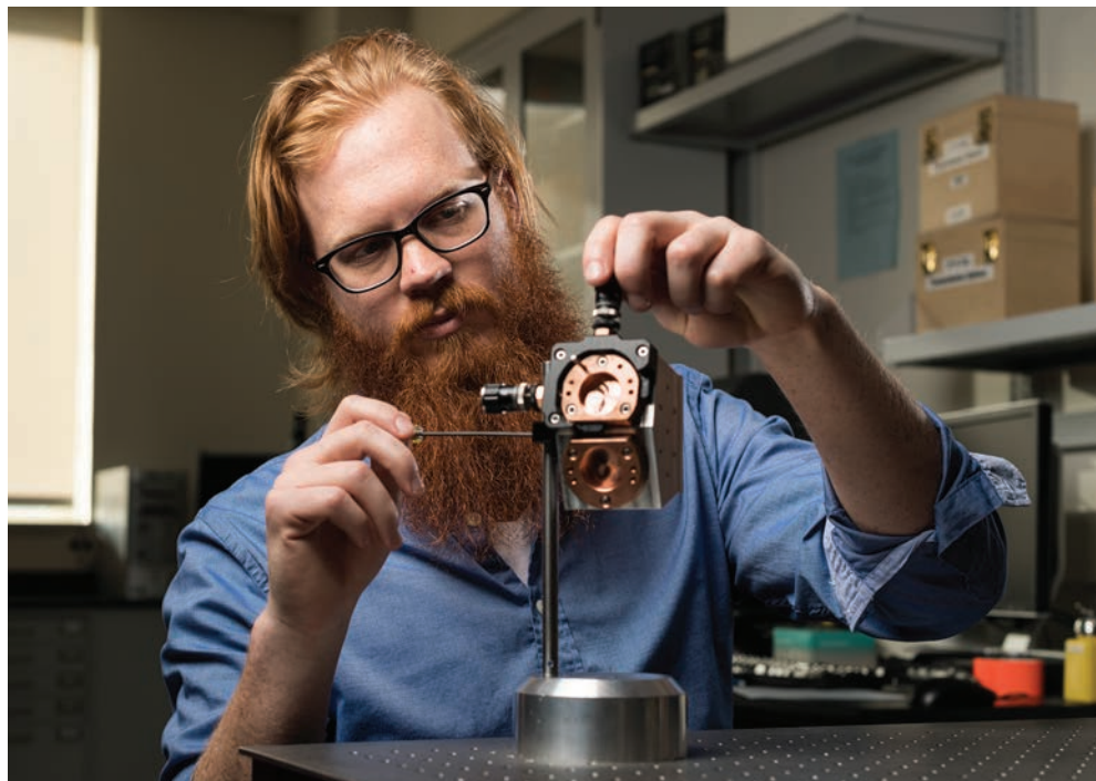
DECENTERED: Designed with freeform optics, Reimers’s prototype spectrometer is lighter, more compact, and more efficient than traditional spectrometers.
