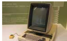
$32,000 PERSONAL COMPUTER: Accompanying the Alto's sleek desktop setup was a processor box that fit in a small metal cabinet.
